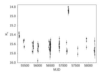
**Figure B1.** VVV  $K_s$  light curve for the submm-bright source VVV J161053.93-515532.8. A jump of  $\sim$ 0.9 mag occurred in mid-2015, lasting for at least 13 days and perhaps several months.
