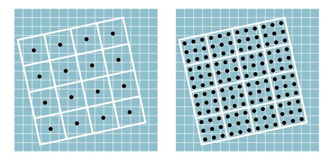
Figure 9: Oversampling in SWARP. The input grid is shown as small grey squares, whereas the output grid (resampled image) is represented by the large tilted ones. *Left*: Without oversampling, only one interpolation (dark spot) of the input image is done at the center of each output pixel. *Right*: with oversampling, several interpolated samples are obtained on a regular subgrid, and then binned in each output pixel. Here a  $3 \times 3$  oversampling is sufficient.
